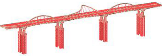
图 7 整体二阶失稳模型 Fig.7 Overall second-order instability model
