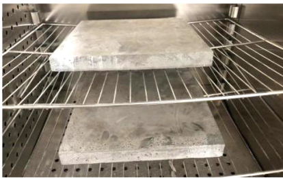
图 6 导热系数测试试块烘干 Fig.6 Drying of test block for thermal conductivity test
