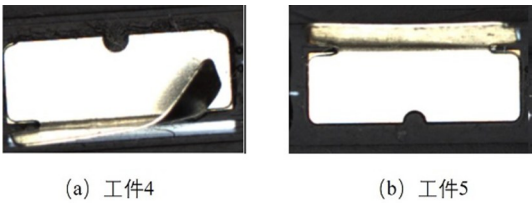
图 9 缺陷工件实物图 Fig.9 Physical drawing of defective workpiece
