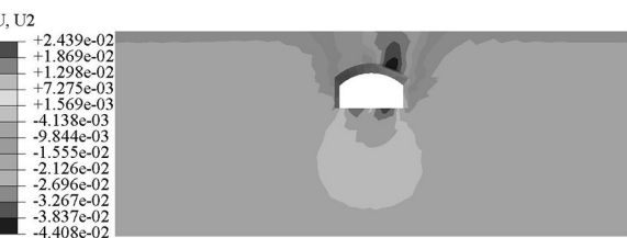
图 9 风险因素作用下 CRD 法沉降云图(单位:m) Fig.9 Settlement cloud map of CRD method under the action of risk factors(unit: m)
