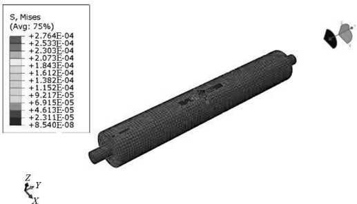
图 6 30 mm 灌浆缺陷工况下的应力云图 Fig.6 Stress nephogram of the condition with a 30 mm grouting defect
