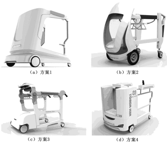
图 1 组新型康复训练机器人设计方案 Fig.1 Four design schemes of new rehabilitation training robots
