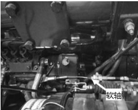
图 3 油门软轴图 Fig.3 Diagram of the throttle shaft
