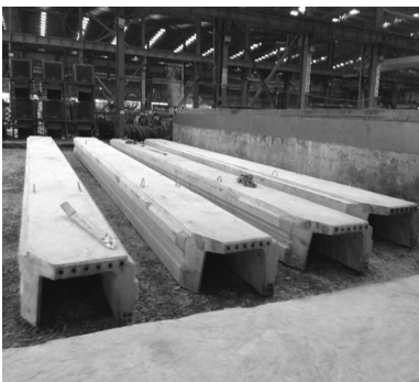
图 1 高强预应力混凝土槽形板桩 Fig.1 High-strength pre-stressed slotted concrete sheet piles
