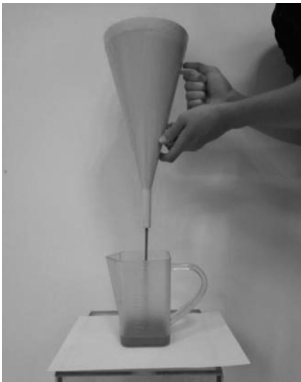
图 2 泥浆 Fig.2 Funnel viscosity measurement of slurry
