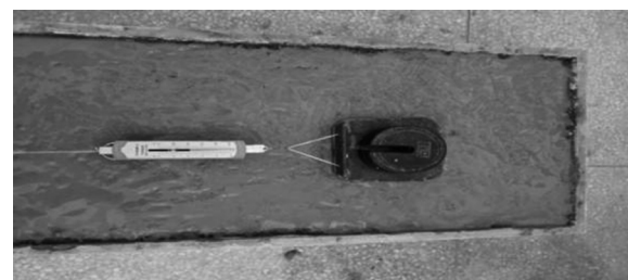
图 10 不同配合比泥浆下砂土与钢板的摩擦系数测定 Fig.10 Determination of friction coefficients between sand and steel plate under the action of slurries with different mix ratios
